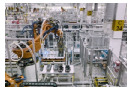
FAW-Volkswagen Smart Workshop's Automatic Battery Assembly Line
